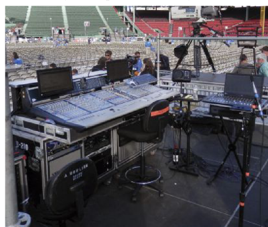
Scovill's front of house cockpit in full, with the VENUE D-Show console joined by an Avid S3L modular mix system at right.
